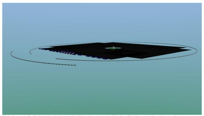
This image of a Solar Island shows the PV solar array in black, with the wave break as a ring surrounding the facility.
